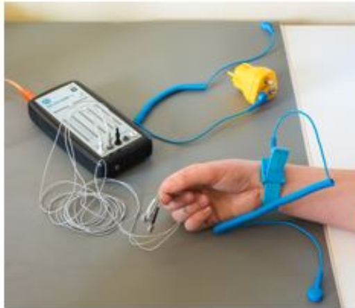
Fig. 2: Antistatic mat and ground strap are connected together via a special plug to the ground of the household power grid.
